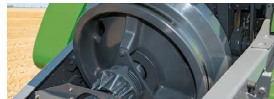
The 545 kg flywheel enables uniform and smooth running, while ensuring high power transfer.
